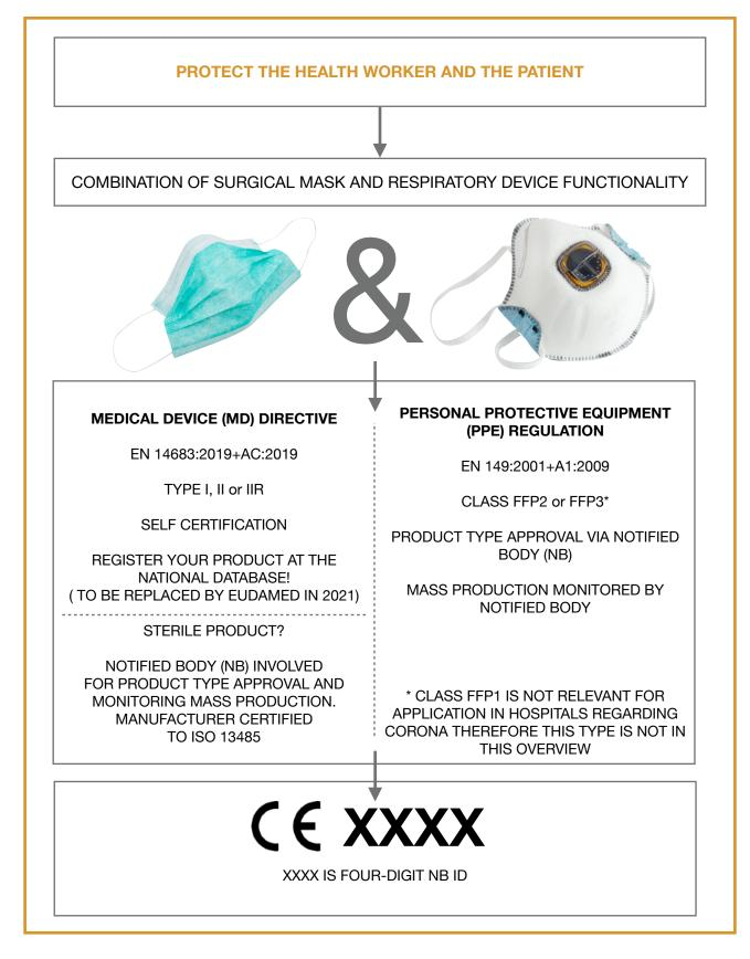
Asking the question "Medical or not?" is ultimately incorrect, as both masks (SURGICAL MASKS approved to EN 14683 as well as RESPIRATORY PROTECTIVE DEVICES approved to EN 149) have suitable application in hospitals. So what is going on? An overview!
